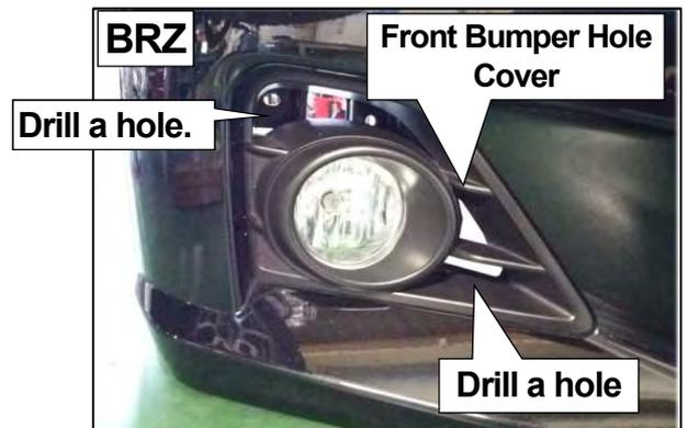
(13) Drill an 8mm hole in the position shown in the diagram on the right. Relocate the washer inlet.
